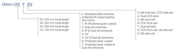
e.g Omni-\(\lambda\)3047, side entrance, slit front exit, slit side exit, support 3 gratings simultaneously, UV monochromator.
