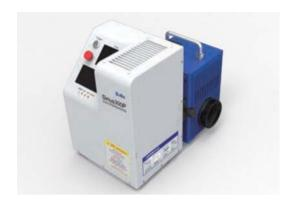
Sirius-300P series photocatalysis light source has high output from UV to NIR, Sirius-300P-F focus on simulated sunlight of visible light; Sirius-300P-UV has strong continuous output within 200-400nm and focus on applications of high UV requirements. Spectral curve as right picture:
