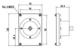
Both are enclosed in a housing with BNC signal connector, and include mounting flanges for the direct mounting on the slit assembly of Omni- $\lambda$  series monochromators. I-V amplifier ZAMP is recommended for the signal conversion
