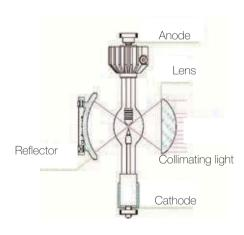
500W Arc light housing expand to operates 350 W Xe and 500 W Hg(Xe)arc lamps under optimal and for these lamps necessary conditions. Switching between the lamps only requires changing the lamp adapter to position the lamp in the center of the housing.
