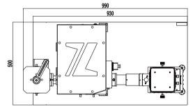
This system adopts the wide band wavelength tunable monochromatic light source and integrating sphere, up-looking configurations (8° focusing). Sample stage is 160 \* 160 mm, convenient placement of all kinds of plane object for testing, such as all kinds of functional fabric. At the same time, the system integration of the transmittance measurement probe, can measure all kinds of pervious to light material (thickness less 5 mm).
