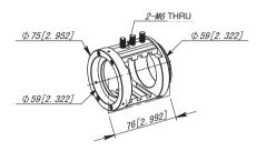
These holders are open to allow easy access to the filters. You can insert various round or square filters simultaneously.
