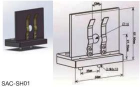
standard sample holder, which can hold sheet solid and liquid (need cuvette)
