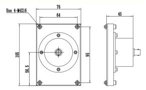
DlnGaAs series Detectors are room temperature, high performance. InGaAs detectors operating over the NIR range from 0.8µm to 2.6µm. The two kinds of DlnGaAs1700-R03M, DlnGaAs2600-R03M detectors have the same construction design.
