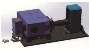
This system adopts the wide band wavelength tunable monochromatic light source and integrating sphere, downlooking configurations, sample stage for small drawer sample box, convenient to place the powder samples, easy to replace.
