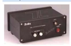
Zolix offers a variety of low noise, high gain amplifier to working with the single channel detectors. The amplifier is mainly used to convert detector output signals, and amplify the signals. Then the signals are inputted to other measurement equipments, such as data acquisition system, oscilloscopes, DMM, to achieve weak signal measurement.
