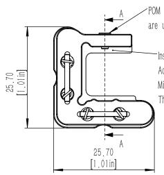
POM glue head screws are used to fix optical elements.
