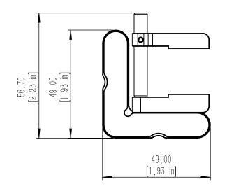
Suitable for cylindrical optics, left hand Components up to 32.0 mm [1.26 in]. (excl. optical elements)
